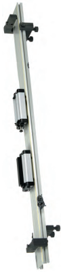
Figure 4.2 Low-friction track and carts used in the experiments described in this chapter.
